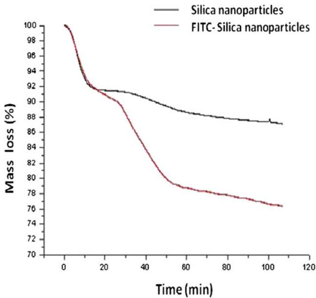
**Fig. 3** TGA curve of FITC-SNPs and SNPs (*Red line* denotes the TGA curve of FITC-SNPs and *black line* denotes TGA curve for bare SNPs)
